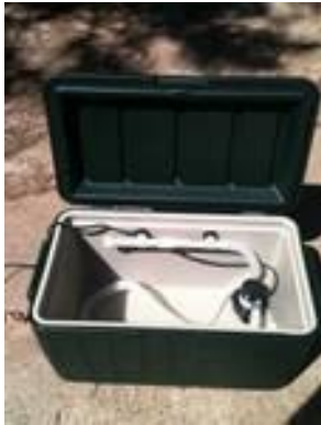
The cooler with the aerator pump and hose attached.
